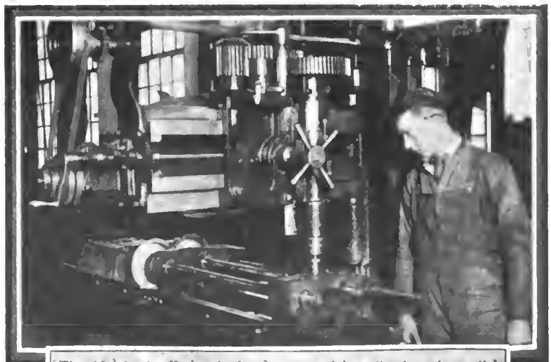
Fig. 16—At the National, showing a special application of a radial drill, with a special fixture, boring three rows of bearing holes at one time
